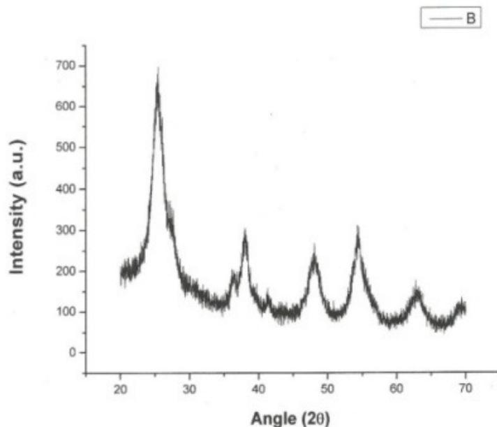
**Figure 1.** X-Ray diffraction pattern of TiO<sub>2</sub>- nps dried at 120<sup>0</sup>C
