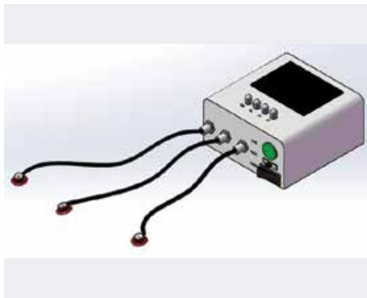
Figure 1 CAD Design of the heart murmur detector
