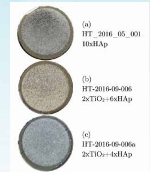
Fig. 2. Deposition difference when applying TiO 2 as a bonding layer before HAp deposition. (a) No TiO 2 applied as bonding layer and 10 layers of HAp, open coating in the upper left corner (b) 2 layers of TiO 2 prior to 6 layers of HAp, closed coating (c) 2 layers of TiO 2 prior to 4 layers of HAp, closed coating.
